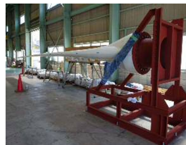
Prototype of innovative stall control blade of a Wind Turbine made in collaboration work
