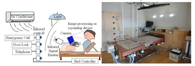
A feature of the support system is that all the machines and electric appliances are connected with the computer via infrared signals. Due to this feature, the computer is free from bothersome cables.
