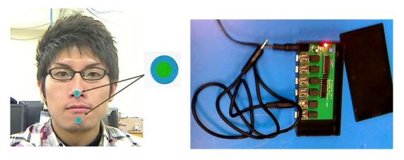
We propose a computerized environment as shown in Figure 1. The system is composed of a vision input device, an infrared signal emitter and infrared controllers. The infrared signal emitter can control electric appliances like TV, air-conditioning system and light. The infrared signal emitter also can control other devices and machines via the infrared controllers. The infrared controllers can control the devices and machines based on the infrared signal detected.
