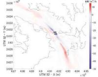
Current velocity measured in the wake of a 0.5 MW tidal turbine
